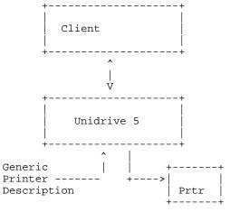
The OS uses the GPD to dynamically build the UI for the printer based upon the device options, constraints and other information provided with the printer and information provided at install time. The GPD syntax has the ability to include macros which can be called to set a group of setting to achieve some singular purpose (fastest, best quality, etc.)
